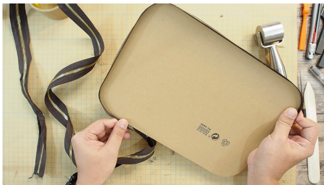
Glue "Stiffener" to top and bottom of "cushion"
